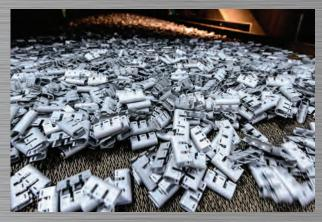
Our advanced dip-spin applications ensure consistent, precise coating thickness on simple to complex metal parts.
